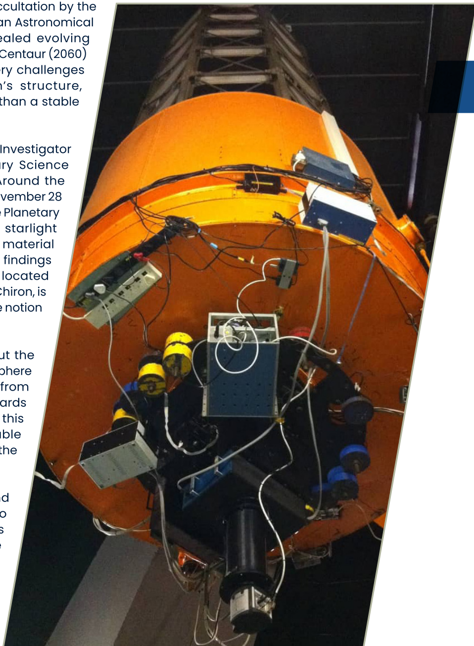
Image: The 1.9-meter telescope at Sutherland, South Africa, shown from the base, with the SHOC (Sutherland High-Speed Optical Camera) instrument. Amanda Sickafoose was the Principal Investigator in the project to build SHOC using a grant from the S. African National Research Foundation. Credit: A. Sickafoose/PSI.
